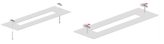
Tighten Spring Toggle until it has just threaded onto screw
