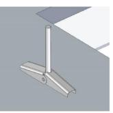
Ensure Spring Toggle is firmly secure into Ceiling Tile
